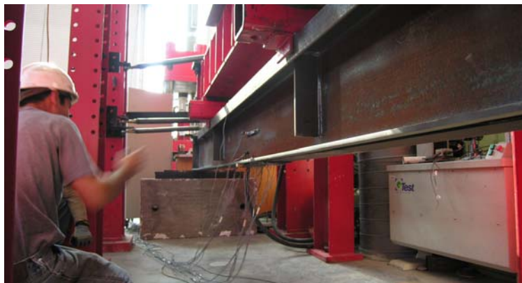
Figure 1: Steel splice beam test
