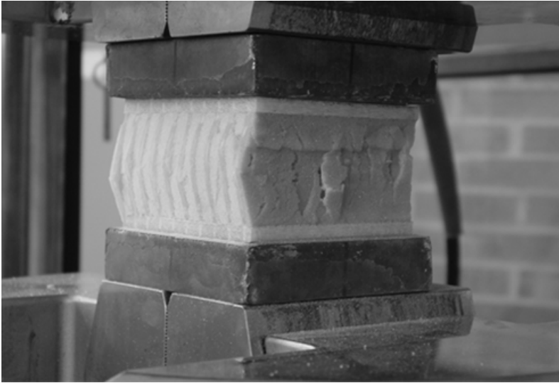
Figure 16. Buckling of through thickness fibers at failure
