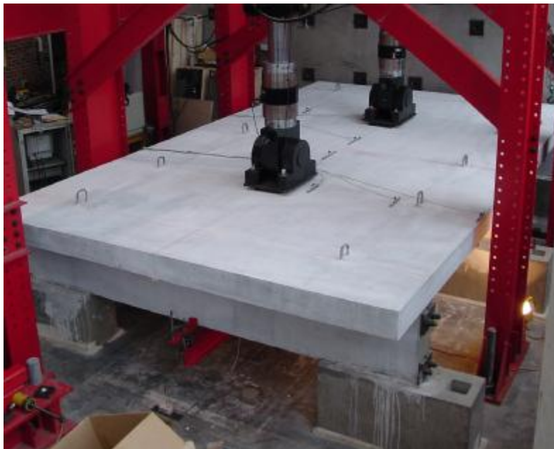
Figure 1: Full-scale bridge deck reinforced with MMFX steel
