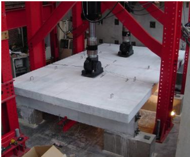
Figure 1: Full-scale bridge deck reinforced with MMFX steel
