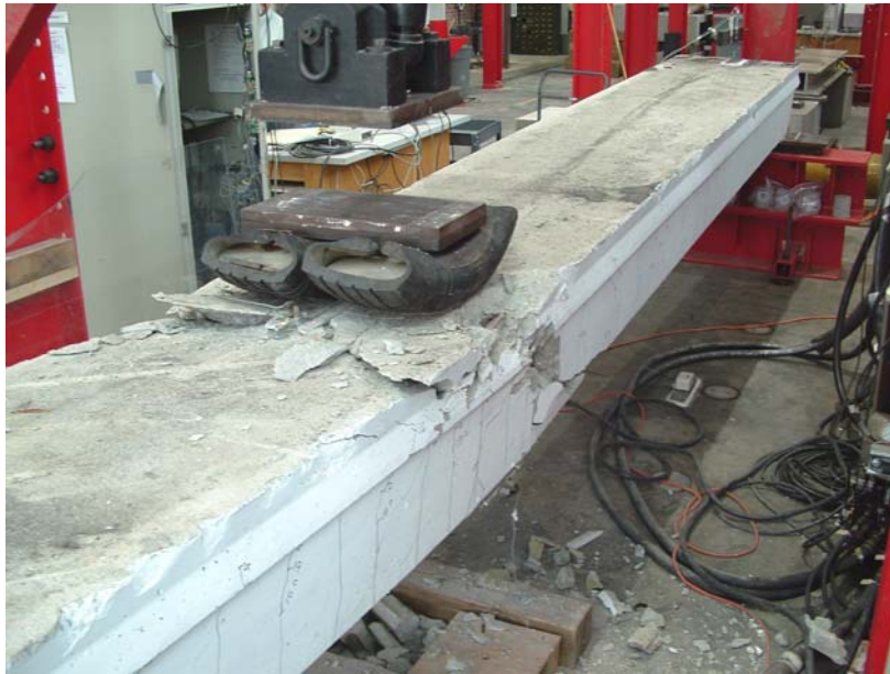
Figure 5. Typical failure due to concrete crushing for the NSM strengthened specimens
