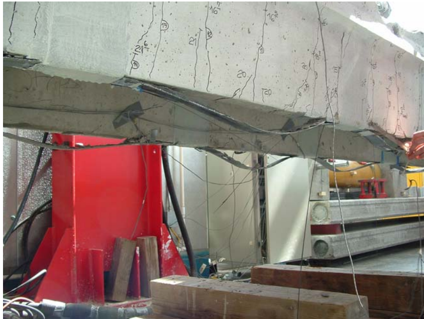
Figure 6. Debonding failure of externally bonded strips in girder S3
