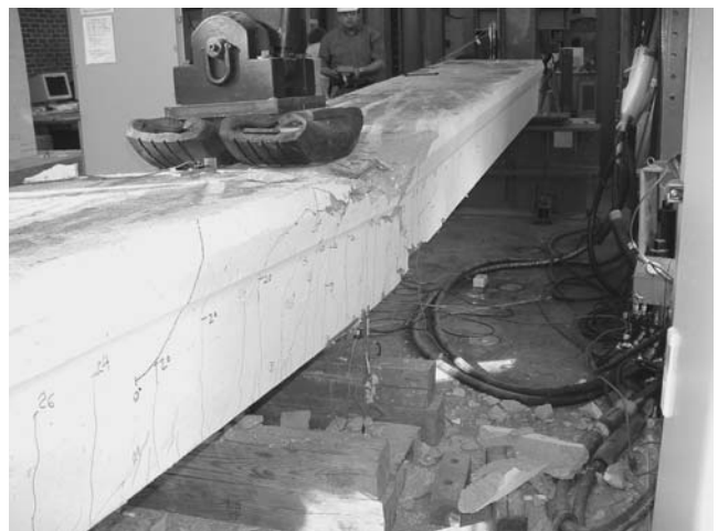
Figure 5. Typical failure due to concrete crushing of the specimens strengthened with NSM CFRP systems
