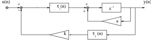
**Figure 2:** Proportional feedback control of a first order discrete time system via a data communication network
