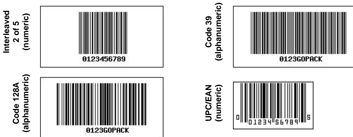
Figure 47. Bar codes used in warehousing. 6
