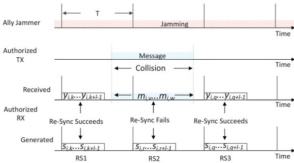
Figure 8. Transmission detection and recovery under ally friendly jamming. The authorized RX and the ally jammer are both in  $i$ -th epoch.  $s$  is the regenerated ally jamming signal,  $y$  is the received ally jamming signal,  $m$  is the received collided signal.  $T$  is the re-synchronization interval.
