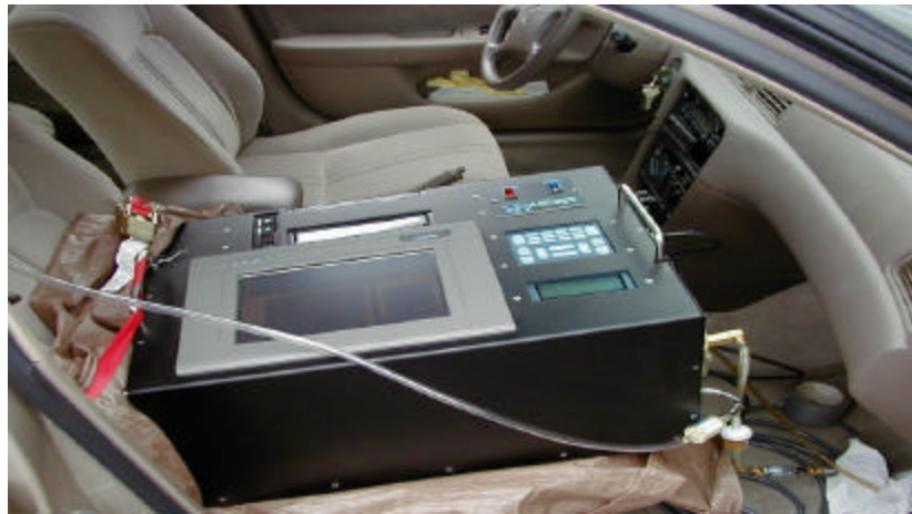
FIGURE 1 OEM 2100 installed in a 1998 Toyota Camry.
