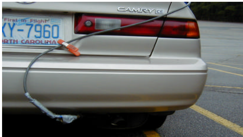
FIGURE 2 Sampling probe routed from vehicle tailpipe into vehicle, secured by clamps.
