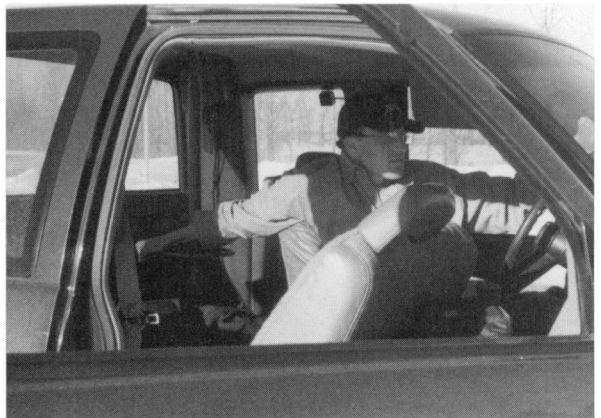
Figure 3. Driver operates mast steering wheel for a vehicle-mounted Null-Peak antenna system.
