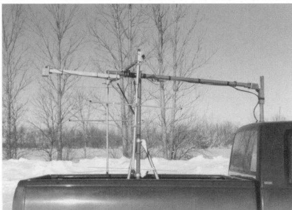
Figure 5. Antenna in folded position rests on a tripod mounted to the bed of the pickup.
