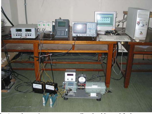
Fig. 3. Actual experiment setup to collect healthy and faulty motor data.
